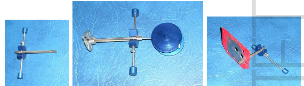
Fig 1. Fortress test lock Fig 2. Fortress internals including curtain Fig 3. Fortress internals including side warding
