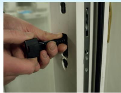
Once the cylinder has been snapped, the lock still needs to be opened, and the cylinder cam turner is the tool to help you do this easily!
